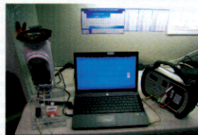
Fig. 9 Thermo Hi-SD XRF spectrometer manufactured by Bruker Corporation. The black octagonal guide table at upper left supports the stamp being analyzed. The instrument at right is a vacuum pump. Courtesy Tom Lera, with permission of the Smithsonian Institution Scholarly Press.
